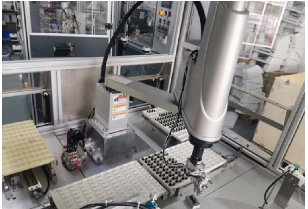
Robot Arm and Vision Inspection System
